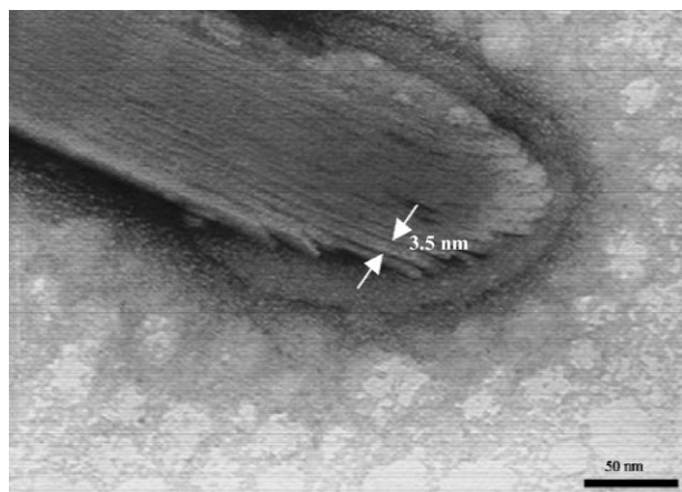
Fig. 2 High resolution TEM image of C20-3'TMP dispersed in deionized water (1 mg ml -1 ). Negative staining ammonium molybdate 1% in water.
